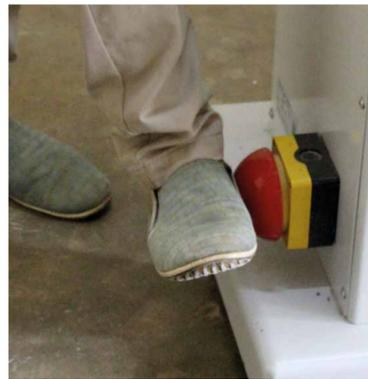
Learn how to stop any machine that you may work on. Keep the floor area around a machine clear and free from obstruction.
