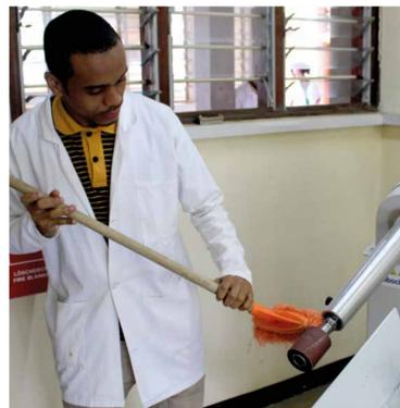
Never clean or adjust machinery in motion. You should never operate any machine unless authorized to do so.
