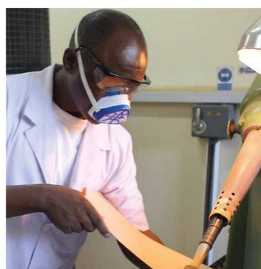
Again, appropriate protective clothing, such as goggles or facemasks, should be worn when operating machines that do not have an integral eye-guard, when grinding plastic materials.
