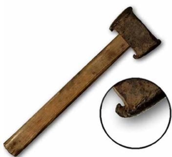
Faces of hammer heads must be kept sound and in good shape.
