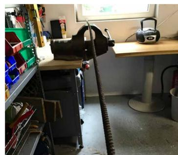
Metal bars or other materials being worked on by hand should not be held in the vice or on the bench in such a way that they project into a pathway.
