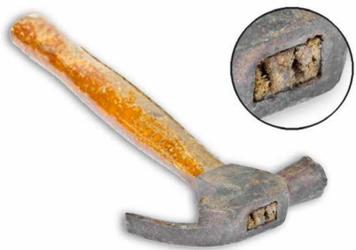
Handles must always be securely fixed, e.g. chisels, files, hammers and planes.
